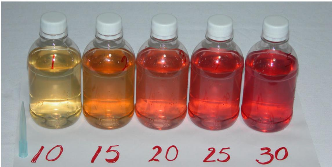
Figure 1: Potassium permanganate (mg/L) demand of raw water
